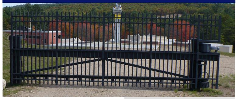
The **SUPER SWING GATE** (SSWG) features a structural steel beam that opens horizontally for crash rated vehicle security. Gate facades include chain link, pickets or anti-climb panels for pedestrians and bike access control. Great for controlled access points with low to medium vehicle traffic, the SSWG can secure multiple lanes of traffic or wide checkpoints up to 30 feet. For longer spans or split traffic situations two single gates can be combined.
